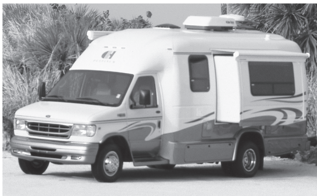
The Platinum 232XL features a slideout that allows the power sofa to fold down without taking up the aisle.
